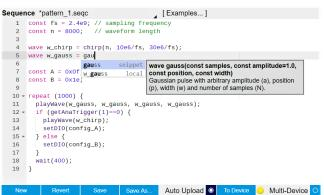
The LabOne UI is designed to get you going quickly by providing hardware control in an intuitive and easily readable form. After defining the waveforms and sequences in the LabOne AWG Sequencer, the LabOne AWG Compiler translates it into machine language and transfers it to the hardware in a minimum amount of time. LabOne sequencing supports loops with dynamically varying delay and conditional branching points.
