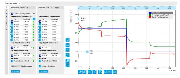
The Precompensation tab in the LabOne UI provides a simulator to display the effect of imperfections of the transmission lines and how to compensate them. Then the correction parameters can be easily transferred to the device.
